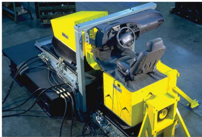
Vehicle Vibration Simulation System (VVSS).
