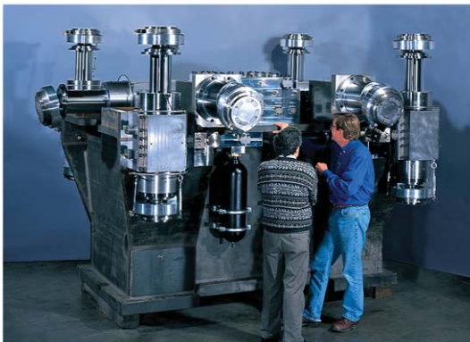
A seismic test system nears completion. Team has designed and manufactured multi-axis test systems for a wide range of applications.
