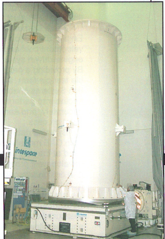
Completed 3 m x 3m slip table shown with test payload. (Photo courtesy of SEREME and Intespace)
